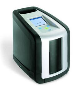
The driver will swab the inside of their mouth, the process usually takes 30 to 60 seconds, although it has been known to take up to 4 minutes. Once sufficient oral fluid is obtained, the swab will be inserted into the main device which will be kept in the police vehicle. Results of the analysis will be available in approx. 4 minutes.
